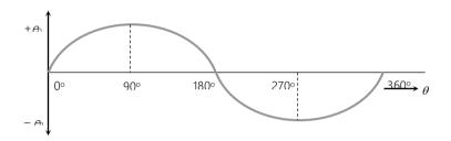
Frequency of ac produced given by  $[f_{AC}] = \frac{NP}{2}$ , where P = Number of magnetic poles of field, N = Rotational frequency of armature coil in rps (rotations per seconds)
