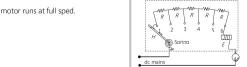
The value of starting resistance is maximum at time t=0 and its value is controlled by spring and electromagnetic system and is made to zero when the motor attains its safe speed.
